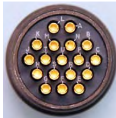
Wiring Side - Solder Cups
