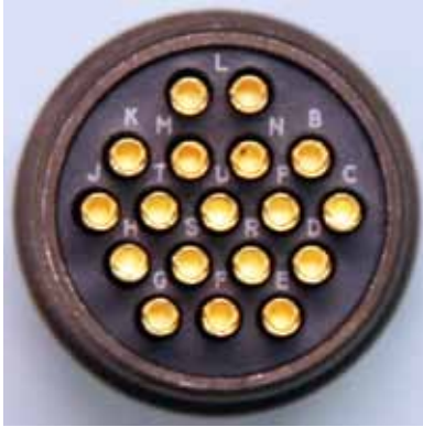
Wiring Side - Solder Cups
