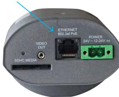
**Direct Power:** Connect either a 12-24VDC or 24VAC power source to the camera. Wire polarity is not important, therefore + or - connections can be connected to either terminal as shown in Figure 2.
