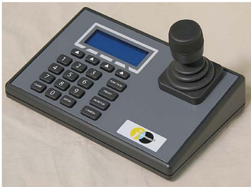
Figure 1. Model 9210 Control Panel
