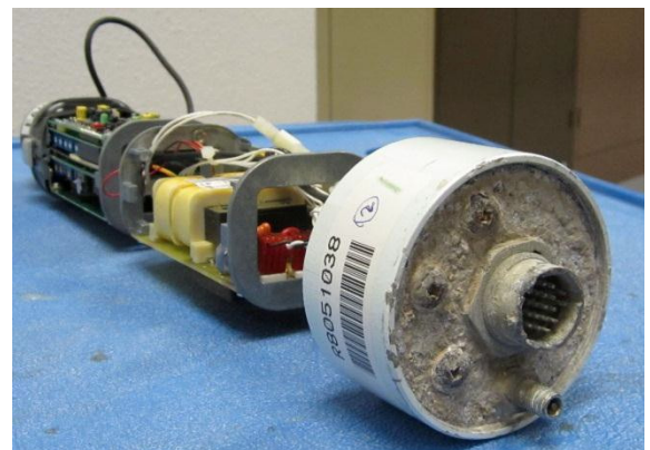
Figure 1 CohuHD 4830 camera with the enclosure removed. Notice corrosion on the outside of the rear plate. However, the optics and electronics inside are pristine.
